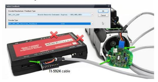
2. Read the memory data and program new alignment angles with TI-5040 (rev C) and TI-5104 module. Disconnect the green resolver connector from the PCB as shown below. The Memory Test button will read the memory data. The Memory Program allows you to write data and program new alignment angles (electronic alignment) as shown in the video titled TI-5000JX Hiperface and Indramat Electronic Alignment.
